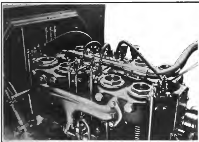
ROCHET-SCHNEIDER MAKE-AND-BREAK IGNITION MECHANISM. NOTE TAPPETS OPERATING IGNITERS.
